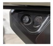
Disengage the kickstand, grab the brake handle to engage the brakes, and seat yourself on the Super73. Switch the battery to the "I" position to turn the bike on. Once the display screen is illuminated, the throttle is active and you're ready to ride.
