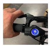
The brake levers are equipped with brake sensors that cut power to the motor when either of the levers are compressed. The ZX employs the Tektro mechanical brake systems. The right lever will activate the rear brakes when compressed and the left lever will activate the front brakes when compressed.
