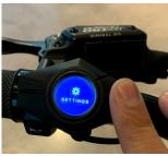
Hold down the "O" button on display to activate the settings menu. Settings parameters:
