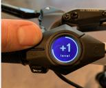
To select your pedal assist mode, follow these steps once the display has been turned on and you are seated on the Super73: Press on the menu "O" button briefly to switch between display views until "Assist" appears on the screen.
